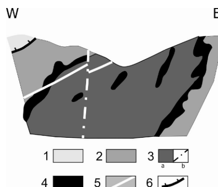
Figure 10. Suvorov – Moldova Noua Cu skarn-porphyry deposit (adapted from [18]) 1. Supragetic crystalline rocks; 2. Mesozoic carbonate rocks converted into marble; 3. Banatites: a) Cu-Mo mineralized quartz diorite porphyry – granodiorite porphyry, partly mined out in open pit, b) post-ore lamprophyre; 4. Cu skarns, mainly mined out in underground; 5. Fault; 6. Thrust
